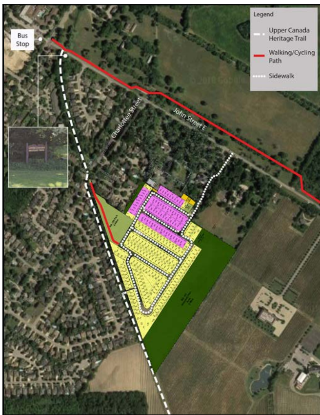
Figure 6. Active transportation opportunities includes sidewalk access to the Heritage Trail and a protected paved cycling/walking path
